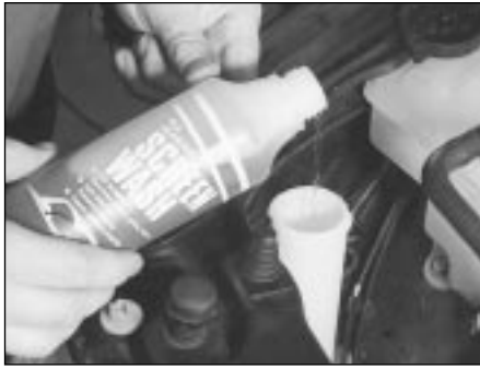
3.17 Topping-up the windscreen washer reservoir
