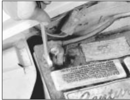
9.6B Removing a lead from the battery terminal - always remove the earth lead first, and connect it last!
