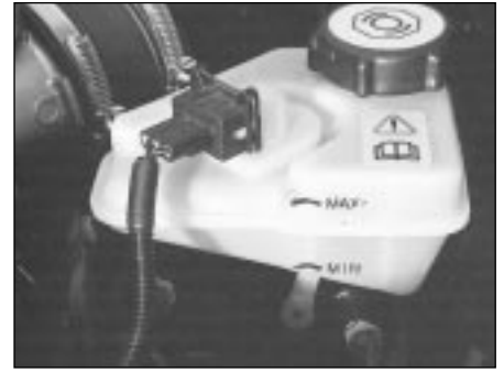
3.19 Brake fluid reservoir, showing "MAX" and "MIN" marks
