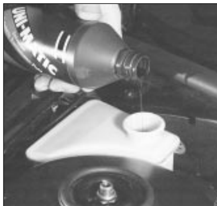
5.6 Topping-up the power steering fluid reservoir
