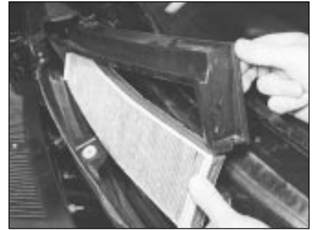
27.5B . . . then withdraw pollen filter element
