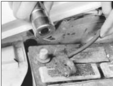
9.7B Regardless of the method used to clean the terminals, a clean, shiny surface should result
