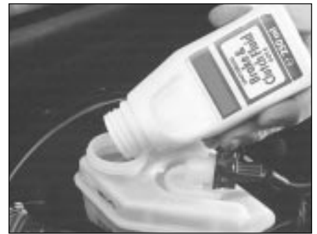
3.22 Topping-up the brake fluid reservoir
