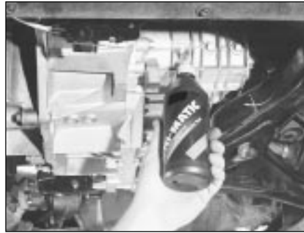
16.2 Topping-up the manual transmission oil
